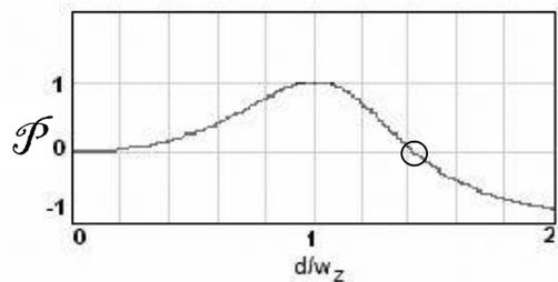
Fig. 7. Radial distribution of the CDP  $\mathcal{P}$  for the combined beam consisting from mutually incoherent, orthogonally polarized modes  $LG_0^1$  and  $LG_1^1$  with the intensity ratio 1:0.45. A circle indicates the  $U$  – singularity position.
