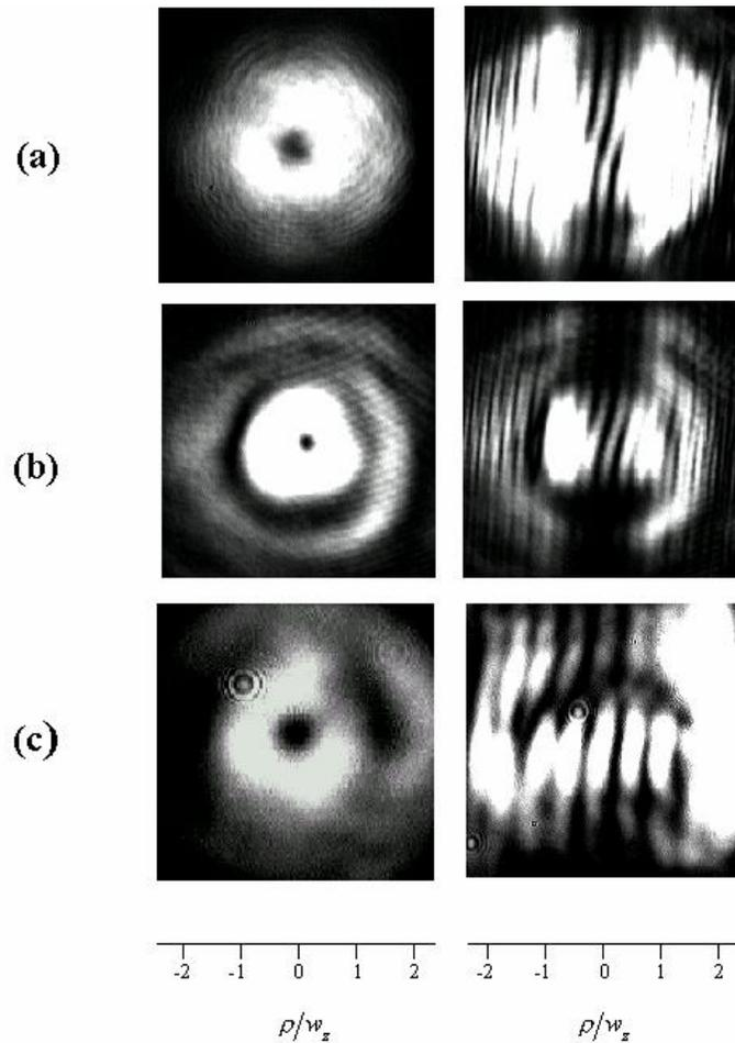
Fig. 5. **a** and **b** – orthogonally linearly polarized Laguerre-Gaussian modes  $LG_0^1$  and  $LG_1^1$ , respectively (topological charge  $m = -1$ ); **c** – combined beam for coherent superposition of these modes observed with a half-wave plate and linear analyzer; right column shows the result of diffraction diagnostics of the central vortex and ring polarization singularity at the ring  $\rho/w_z = 1.45$ .
