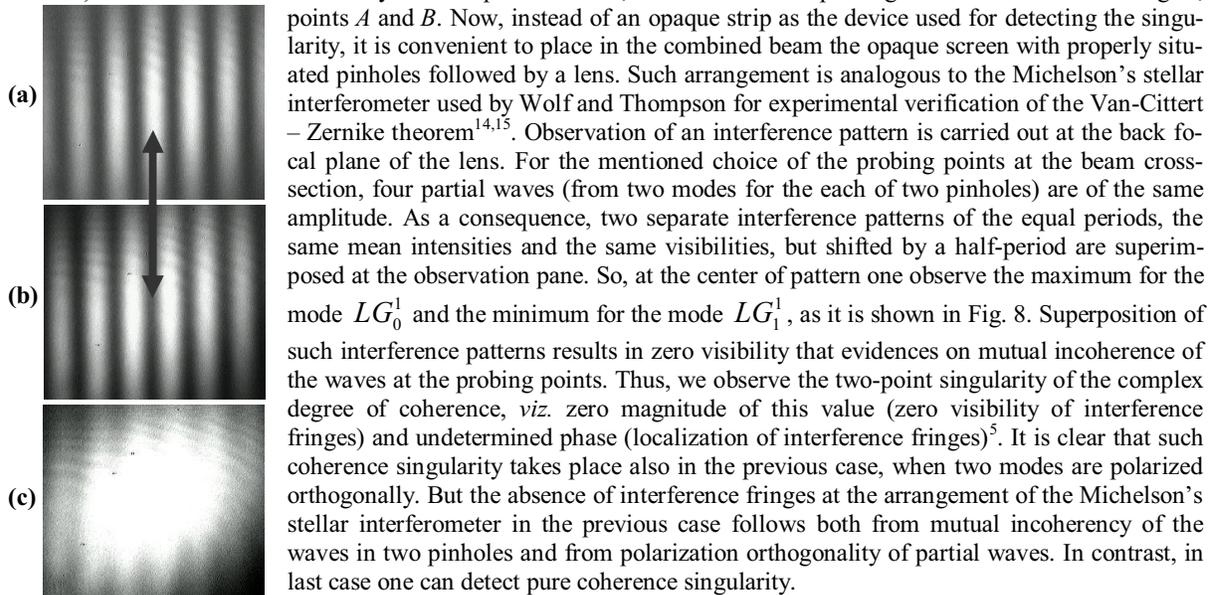
Fig. 8. Detecting the two-point singularity of the complex degree of coherence: **a** and **b** are partial interference fringes for two modes shifted by a half-period; **c** – resulting pattern with zero visibility.
