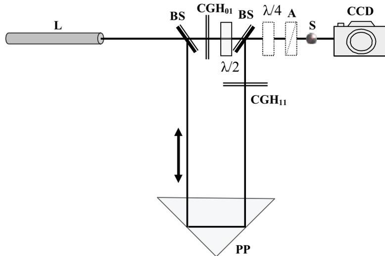
Fig. 1. Principal experimental arrangement for creating the combined singular beam and implementing reincarnation of optical singularities:  $L$  – laser;  $BS$  – beam-splitters;  $CGH_{01}$  and  $CGH_{11}$  – computer-generated holograms reconstructing Laguerre-Gaussian modes  $LG_0^1$  and  $LG_1^1$ , respectively;  $PP$  – Porro prism;  $\lambda/2$  – half-wave plate;  $\lambda/4$  – quarter-wave plate;  $A$  – linear analyzer;  $S$  – opaque strip;  $CCD$  – CCD-camera.
