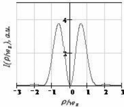
Fig. 3. Radial intensity distribution of the combined beam resulting from *coherent* co-axial mixing of the modes  $LG_0^1$  and  $LG_1^1$  that are in phase at the central part  $\rho/w_z < 1$ . Beside of the central vortex one observes the ring singularity at the ring  $\rho/w_z = 1.45$ .
