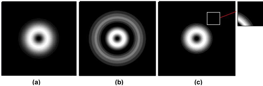
Fig. 4. Constituting modes  $LG_0^1$  and  $LG_1^1$ , **a** and **b**, respectively, and the combined beam. Insert shows a weak side-lobe.
