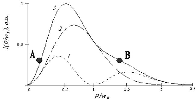
Fig. 2. Radial intensity distributions of isolated modes  $LG_1^1$  (1) and  $LG_0^1$  (2) for the power ratio 1:0.45, and of the combined singular beam (3) resulting from *incoherent* co-axial mixing of the modes.
