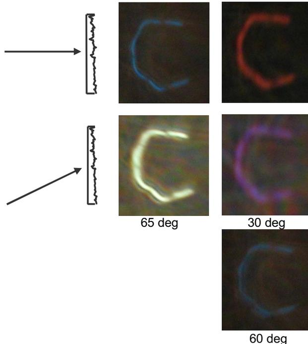
Fig. 9. Dependence of the coloring effect on the inclination of the sample. The upper row show the colors for two specimens for normal incidence of a white-light probing beams, other fragments show changes of colors for the same inclined specimens.
