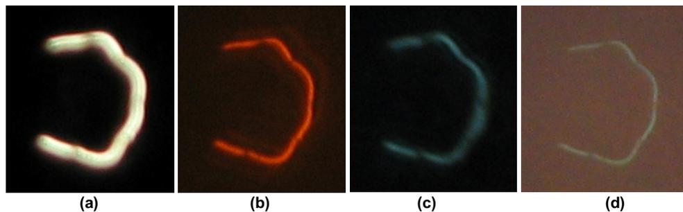
Fig. 6. Lamp filament without diffuser in front of the CCD-camera (**a**), with red-coloring (**b**) and blue-coloring (**c**) *colorless* glasses, and with a sandwich of two similar blue-coloring glasses (**d**).
