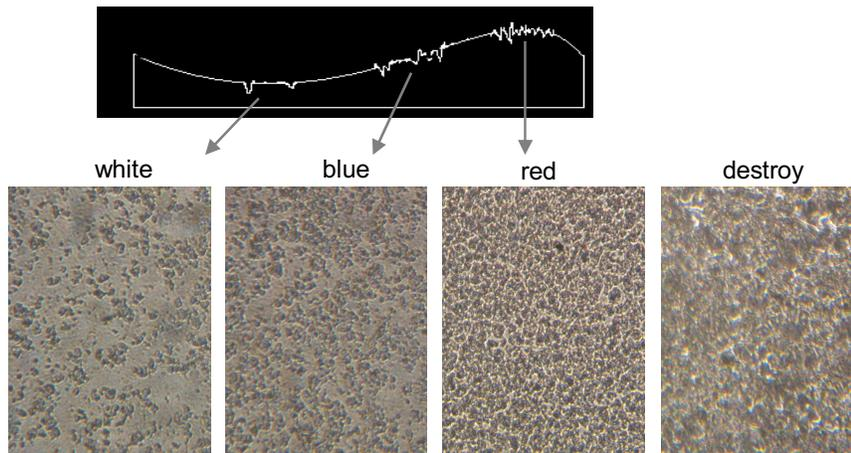
Fig. 5. Topography of intermediately rough surface surfaces inducing coloring the forward-scattered component of a white-light probing beam; the right fragment shows deeply rough surface when the forward-scattered component is completely destroyed.
