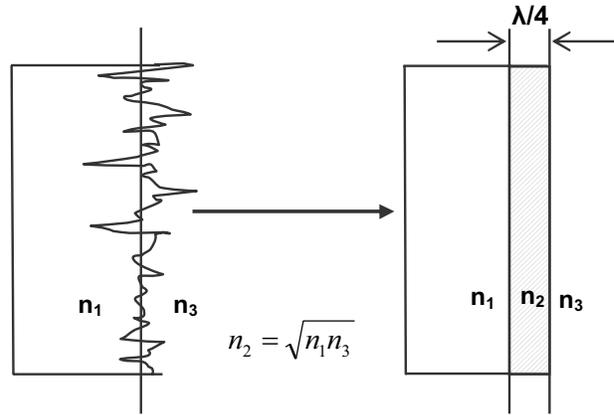
Fig. 3. Analogy between a surface roughness and a transition layer with “diluted” index of refraction.
