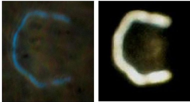
Fig. 8. Dependence of the coloring effect on the position of a rough surface in the imaging system: at the aperture diaphragm (left) and at the field-of-view diaphragm (right).
