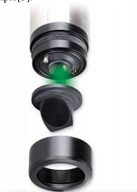
Fig. 5. An example of an optical oximeter.
